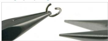
To open a jump ring you will need two pairs of pliers; either flat nose or chain nose pliers. Grab the jump ring in two places near the join using the pliers and twist the ends away from each other. To close the jump ring, twist the ends back together again. Never pull a jump ring apart; it will ruin the tension and shape of the jump ring.
